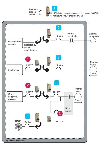
Example of applicable UL 489 circuit breakers and UL 1077 supplementary protectors
