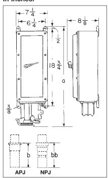
‡Pressure connectors are standard. Crimp/solder type terminators are optionally available for 3 and 4-pole, 30, 60 and 100 ampere. For details, see page 1267. To specify, add the suffix "T" to the catalog number. For example: AP3375-T (Plug).
